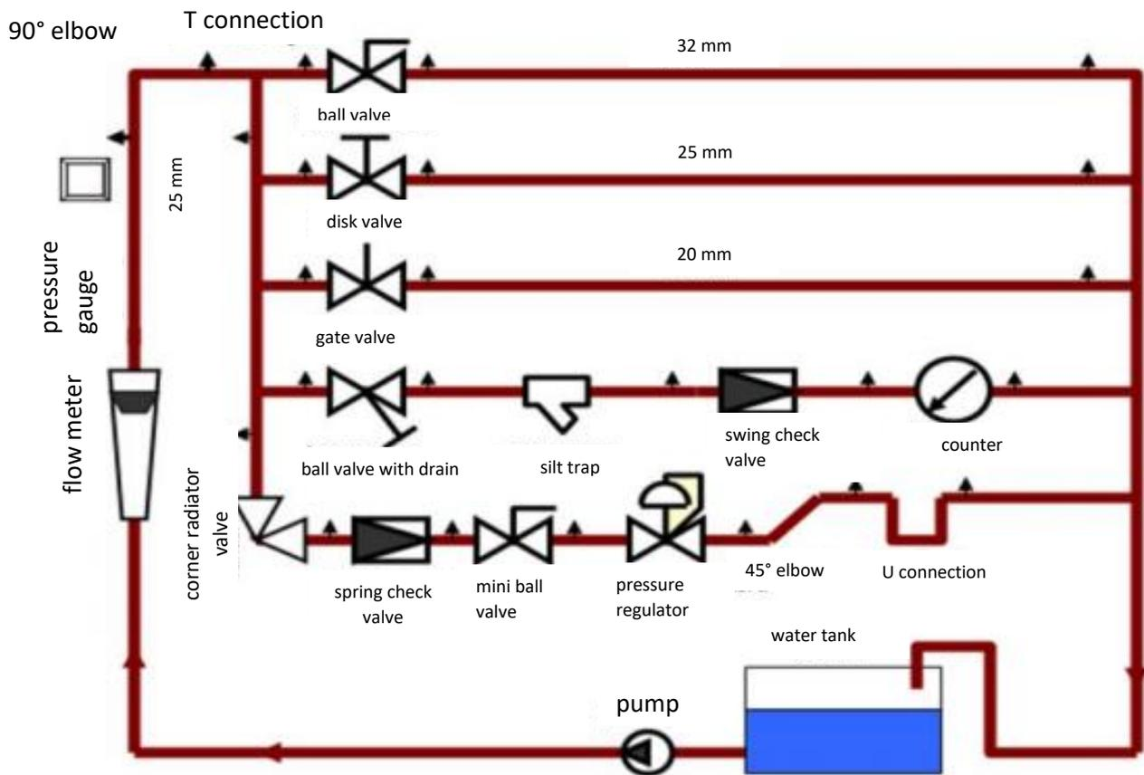
Figure 1. Test system of pressure loss in pipes.
