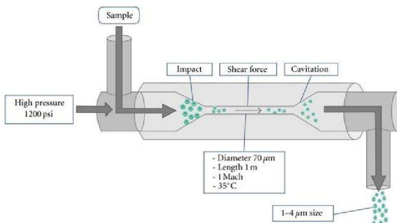
**Figure 4:** A typical high-pressure homogenizer.
