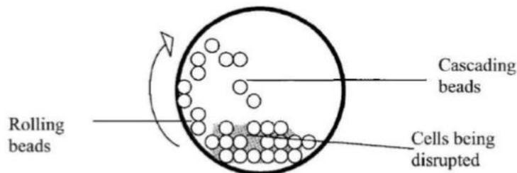
**Figure 3:** The basic principle of a bead mill
